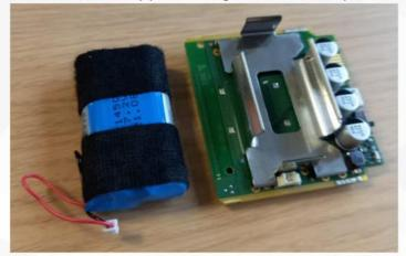
5. Place the new battery back the facing the same direction as previously (cable facing same direction as the red arrow and on the same side as the cable port)
