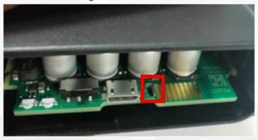
a. First, slightly take it out from the top side by inserting only the tip of the tool (BE CAREFUL NOT TO BREAK ONE OF THE CAPACITATORS)
