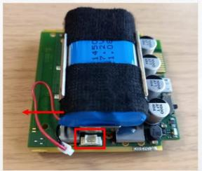
6. Make sure to connect the connector plug with the red wire on the right and the black one on the left.
